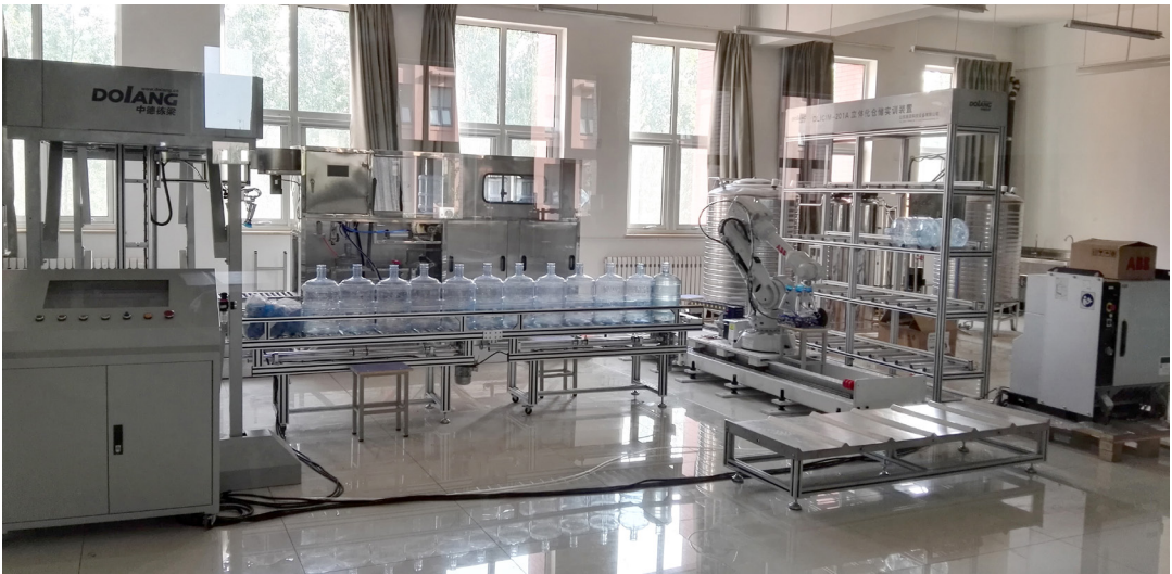
DLIM-201 纯净水自动化生产线实训系统 Pure Water Automatic Production Line Training System
